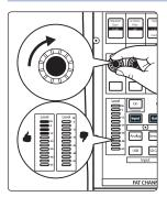
Once the Network input has been selected on the StudioLive Series III console mixer, you can remote control the preamp level and phantom power for your rackmount mixer from the top panel of your console mixer.
