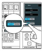
For every channel that you want to source from the Network and record from the console mixer (either USB or SD), you need to set the Digital Send Source to "Digital". To do this, navigate to the channel settings on the console mixer and enable the Digital Send Source.
