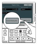
StudioLive Series III mixers route channels in banks of 8. From the Channel Routing page, you can change the default routing:
