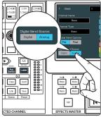
For every channel that you want to source from the local analog inputs and record from the console mixer (either USB or SD), you need to set the Digital Send Source to "Analog". To do this, navigate to the channel settings on the console mixer and enable the Analog Send Source.
