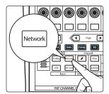
If you would like the input source for any channel on your StudioLive Series III console mixer to come from your StudioLive Series III rack mixer, select that channel on your console mixer and enable Network as the Input Source. For example, if you would like to use the guitar connected to Input 3 on your StudioLive 16R in any mix on your StudioLive 24, you would select Channel 3 on your StudioLive 24 and enable Network as the input source.
